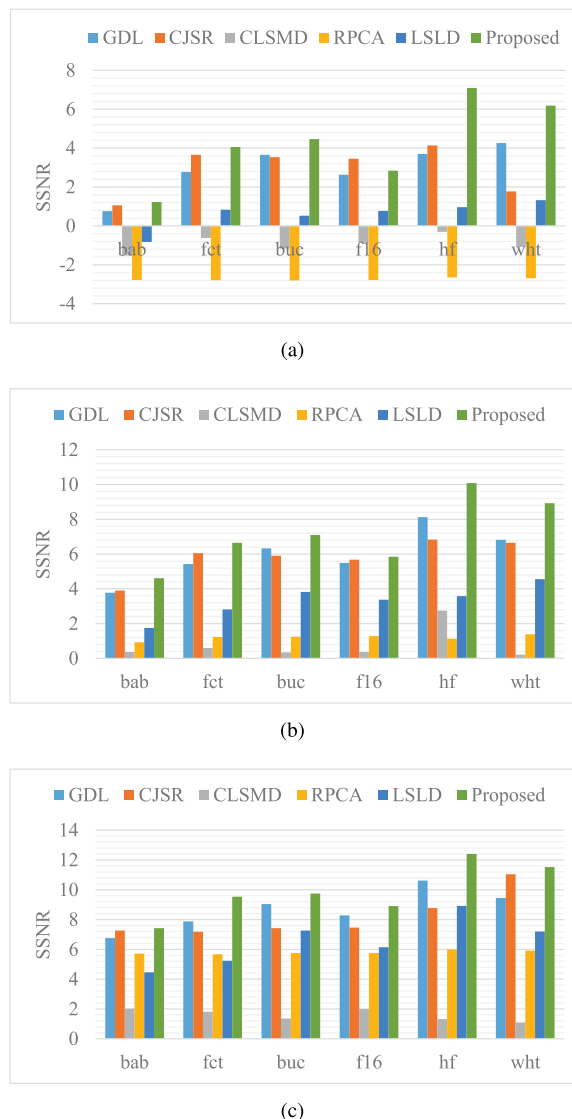
FIGURE 2. Average SSNR results of male speech with six different methods for six different types of noise. (a) SNR=0dB, (b) SNR=5dB, (c) SNR=10dB.
