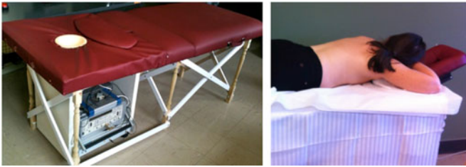
Fig. 2. Patient interface table with measurement system underneath (left) and a patient getting her breast scanned with the system (right) [12].
