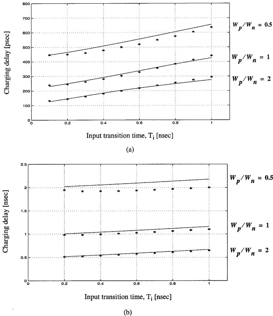
Fig. 7. Dependence of the delay time on the input transition time for inverters (in 0.25- $\mu\text{m}$  CMOS technology) with different transistor-size ratios  $W_p/W_n$  ( $W_n = 4 \mu\text{m}$ ), and for small and large loading capacitances  $C_L$ : a)  $C_L = 150$  fF and b)  $C_L = 750$  fF. Proposed model (\*\*\*). HSPICE simulation: (—).
