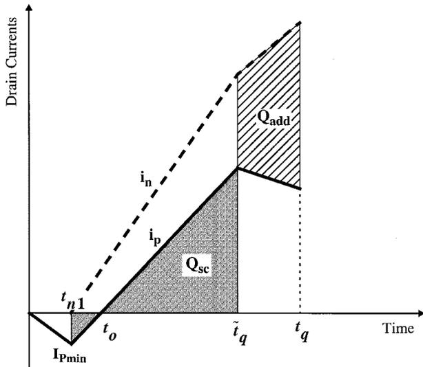
Fig. 4. Piecewise-linear approximations of the discharging current  $i_n$  (---) and the short-circuit current  $i_p$  (—), used in Step 2 of the derivation of the maximum short-circuit current  $I_{P\max}$  for the discharging inverter (rising input).
