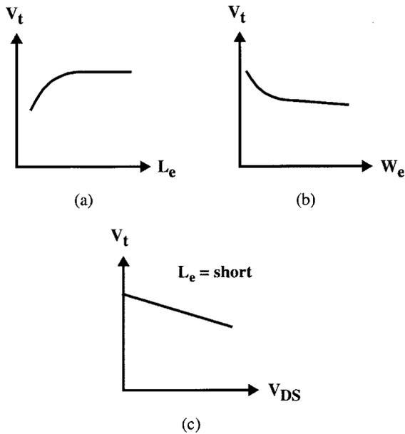
Fig. 1. Sketch of the dependence of the MOSFET threshold voltage  $V_t$  on: (a) the effective channel length  $L_e$ ; (b) the effective channel width  $W_e$ ; and (c) the drain-source voltage  $V_{DS}$  in short-channel devices (drain-induced barrier lowering effect).
