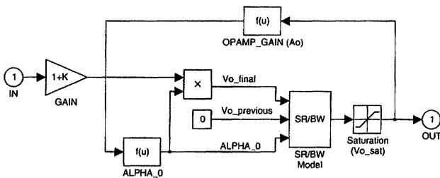
Fig. 4 SIMULINK model of an SC amplifier (Fig. 1a).
