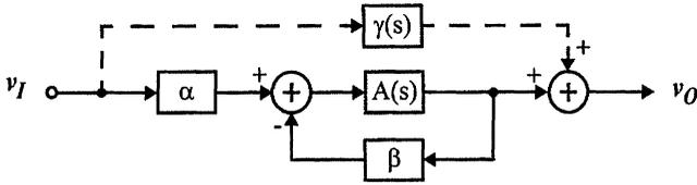
Fig. 2 Equivalent feedback model of an SC stage during its charge-transfer phase (Fig. 1c): a) series-shunt model ( $\gamma=0$ ); b) return-ratio model (forward transmission  $\gamma$  modeled).
