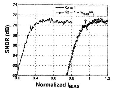
Fig. 8 SNDR vs. normalized bias current  $I_{BIAS}$
