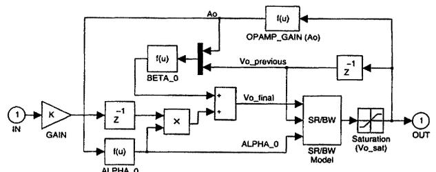
Fig. 5 SIMULINK model of a non-inverting delaying SC integrator (Fig. 1b)
