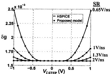
Fig. 6 Gain error vs. input step voltage for various SR values ( $C_S = C_F = C_{out} = 2$  pF;  $C_{in} = 0.2$  pF;  $R_L = 200$  k $\Omega$ ;  $G_m = 10$  mA/V).
