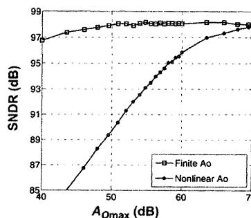
Fig. 7 SNDR vs. maximum dc gain  $A_{0max}$
