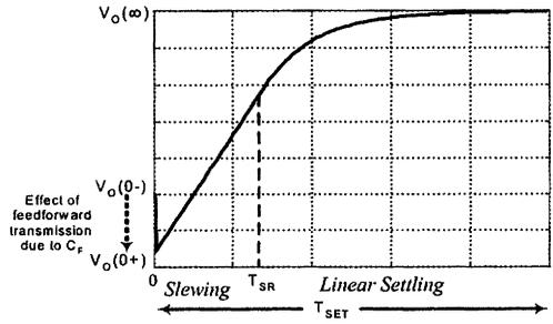
Fig. 3 Typical settling behavior of an SC stage in its charge-transfer phase (Fig. 1c), when a step voltage is applied at its input.
