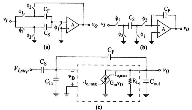
**Fig. 1** (a) SC amplifier; (b) SC integrator; (c) Configuration of (a) and (b) during the charge-transfer clock phase  $\phi_2$ , with the opamp equivalent-circuit model shown. Here,  $C_S$  and  $C_F$  are the sampling and feedback capacitors;  $C_{in}$  and  $C_{out}$  are the total capacitances, including any parasitic, at the opamp's input and output nodes.
