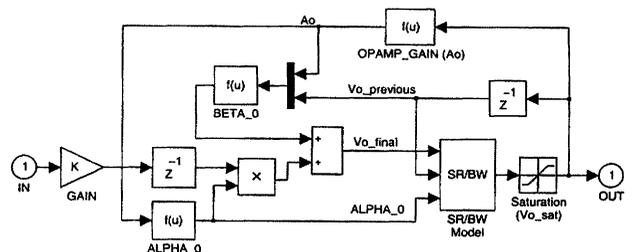
Fig. 5 SIMULINK model of a non-inverting delaying SC integrator (Fig. 1b)
