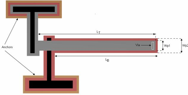
Fig. 2. Schematic view of the proposed double single-beam vertical thermal actuator.
