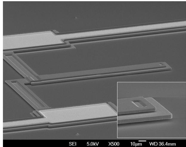
Fig. 7. SEM micrograph of one of the thermal actuators fabricated for testing.
