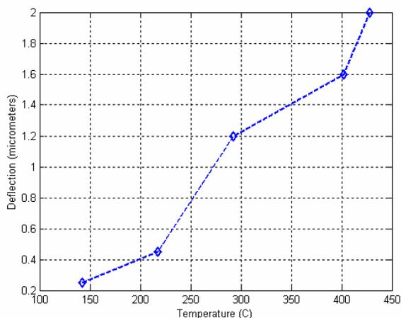
Fig. 8. Displacement of the actuator tip as a function of pad temperature in the direction to the substrate.
