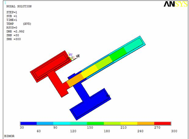
Fig. 6. Numerical results for the temperature distribution of the VTA.
