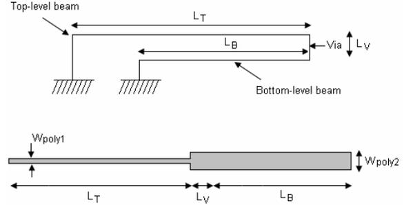
Fig. 3. Simplified coordinate system and diagram of the 'unfolded' actuator of Figure 2 showing the two microbeams connected in series.
