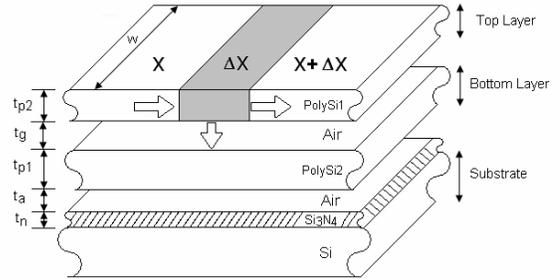
Fig. 4. Cross-sectional view of the actuator's structure.
