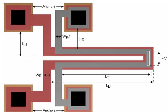
Fig. 1. The classical ‘U’ shape electrothermal vertical actuator.
