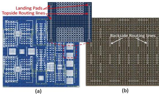
Figure 2. One wafer field design (a) Topside and (b) Backside.
