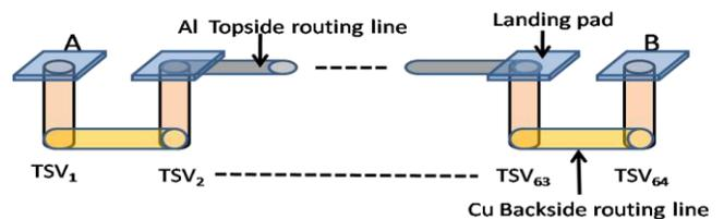
Figure 6. Schematic of TSV chain.
