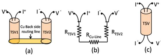
Figure 4. Schematics of resistance measurement (a) the 2-TSV chain test, (b) the equivalent circuit model of (a) and (c) the direct test of single TSV.
