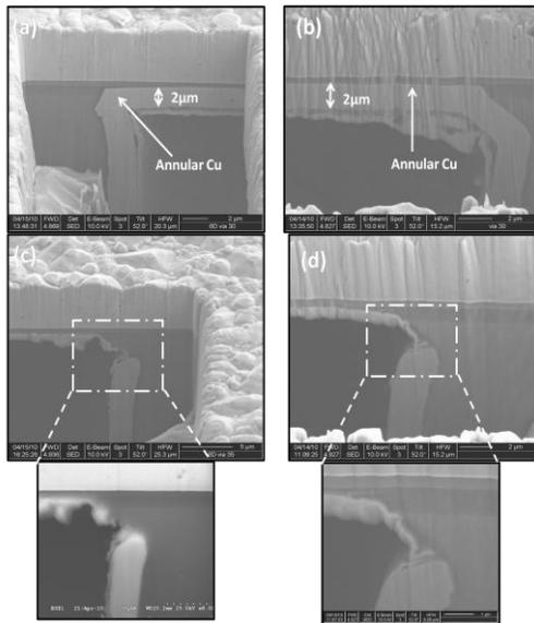
Figure 8. Dual Beam FIB/SEM images inside TSVs (a), (b), (c) and (d) have TSV resistance of 11mΩ, 10mΩ, 6kΩ, and 1.4kΩ, respectively.
