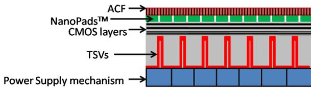
Figure 1. Schematic of WaferIC™ stack.
