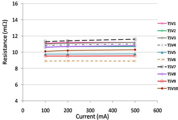
Figure 5. Resistance measurement of different annular TSVs.
