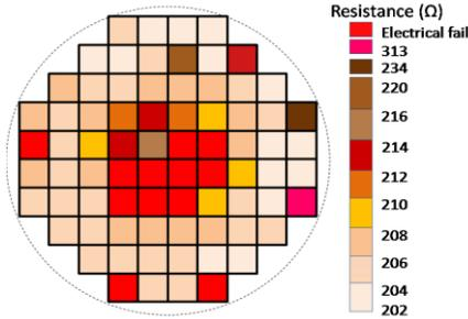
Figure 7. Chain resistance mapping of 76 wafer fields.
