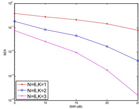
(b) Effects of different number of antennas at relay.
