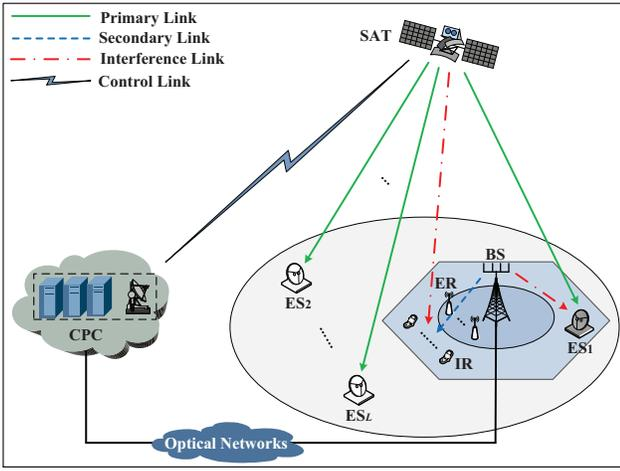
Fig. 1: System model of wireless powered CSTN.
