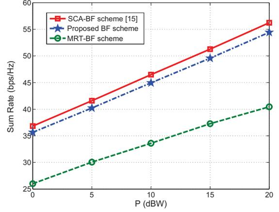
Fig. 3: Sum rate versus transmit power.
