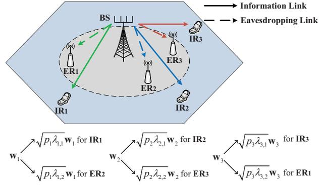
Fig. 2: Illustration of MB-ZF scheme for the case of  $M = K = 3$ .
