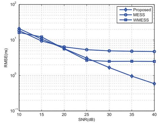
Fig. 1. RMSE of TOA estimator versus SNR for CM1 channel.
