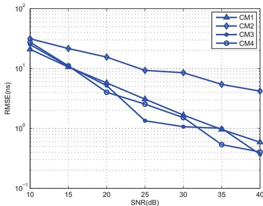
Fig. 3. RMSE of proposed TOA estimator versus SNR for different channels.
