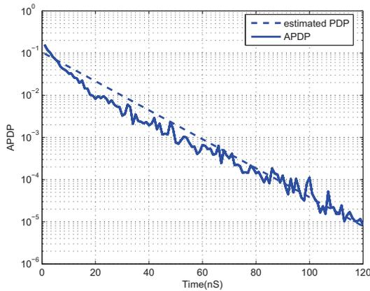
Fig. 2. Estimated power delay profile (CM1 channel, SNR = 40dB).
