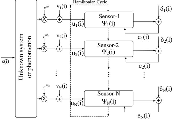
Fig. 1: System model for distributed blind adaptive equalization
