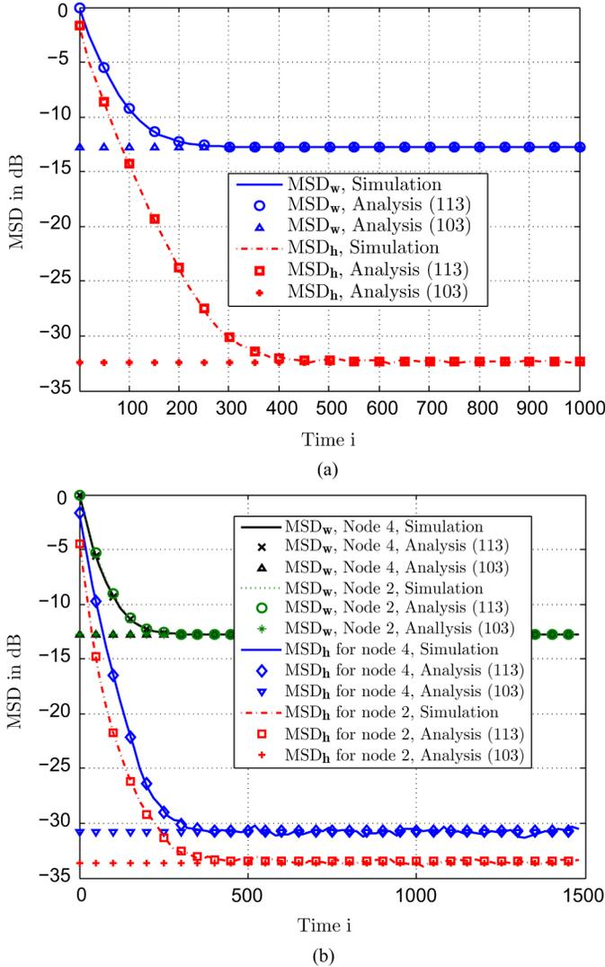
Fig. 2. The network MSD learning curve for  $N = 4$  (a) The network MSD (b) The MSD at some individual nodes.
