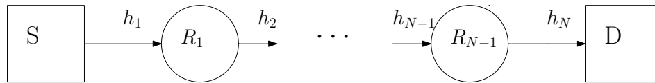
Fig. 2.2: N -hop relay channel with N - 1 single-antenna relay nodes (R) and single-antenna source (S) and destination (D).
