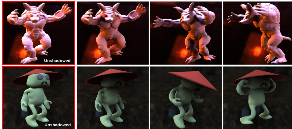
Figure 1: Our system is able to generate PRT coefficients for a dynamically animated character in real-time with a low memory footprint (see Table 2.) Compared to un-shadowed shading using irradiance environment maps (first column), our results clearly improve the visual quality of an animated object. Low memory requirements, fast model fitting and a simple runtime algorithm make our approach suitable for interactive applications, such as games.
