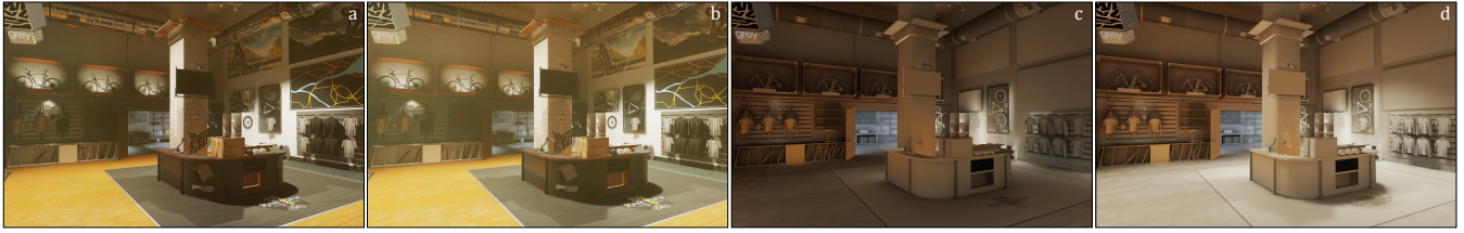
Figure 12: Homogeneous media lit by point and directional emitters. Final renderings (a, b) include scattering towards the eye, lightmap visualizations (c, d) only include indirect light. Only treating directly-attenuated light transport (a, c) fails to capture important volume-to-surface scattering effects. Our method (b, d) accounts for these with minimal overhead, avoiding costly multi-bounce media path tracing. ©Activision Publishing, Inc.
