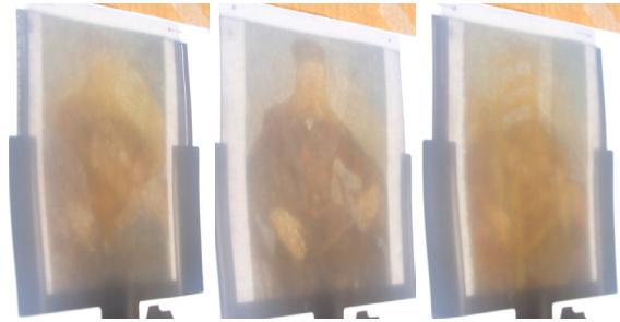
Figure 10: A layered attenuator with only two layers produces three distinct shadows.
