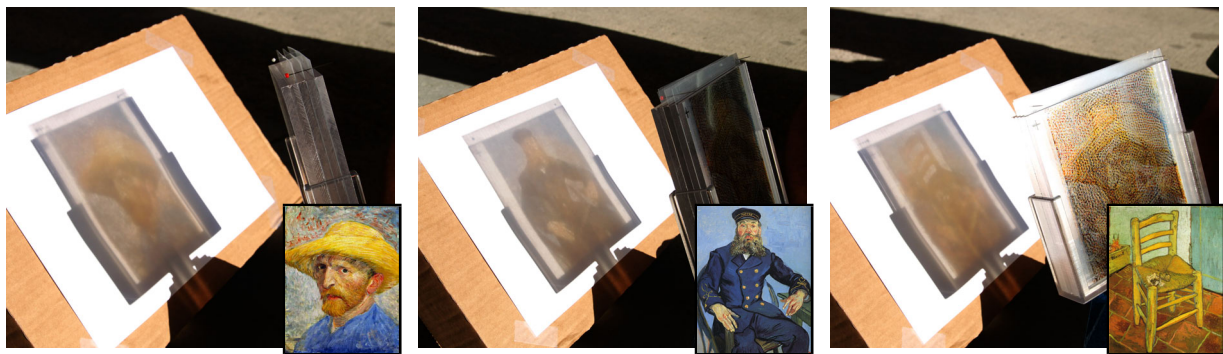
Figure 1: A single manufactured multi-layer attenuator, consisting of three transparencies separated by acrylic, casts different shadows depending on the angle of the sun. The shadows match the target Van Gogh paintings, shown as insets.
