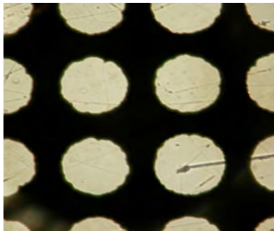
Figure 1: Optical image of backside illuminated TSVs: 200 \mu\text{m} diameter-600 \mu\text{m} thick wafer
