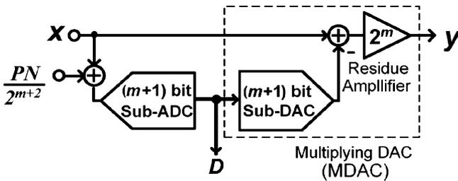
Fig. 4. First pipeline stage (with  $m$ -bit effective resolution) of the  $M$ -bit pipelined ADC in Fig. 1, with a dither signal  $PN$  added at the input of its sub-ADC.
