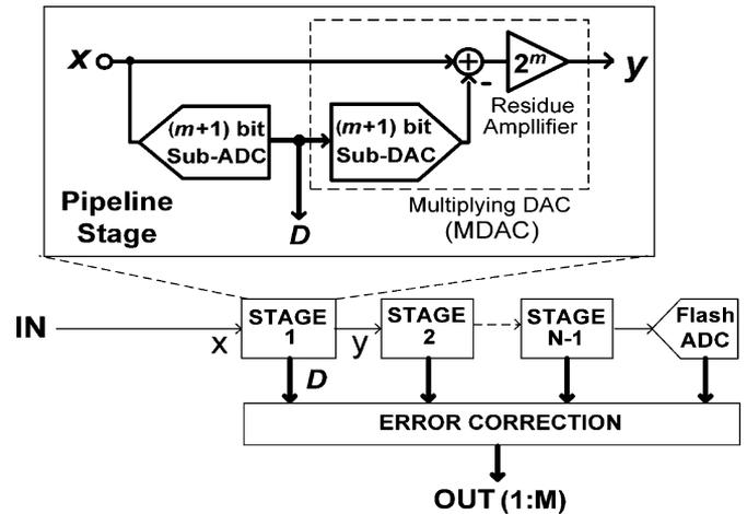
Fig. 1.  $M$ -bit  $N$ -stage pipelined ADC. Its first pipeline stage has an  $m$ -bit effective resolution and a 1-bit redundancy for digital error correction.
