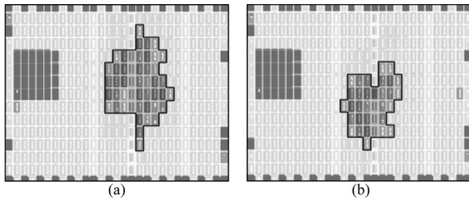
Fig. 7. Area of the calibration unit on the FPGA when synthesized with: (a) full data precision (13 bits) for  $Y$  and  $Y_{PN}$  and (b) precision of  $Y$  and  $Y_{PN}$  reduced from full 13 to 7 bits.
