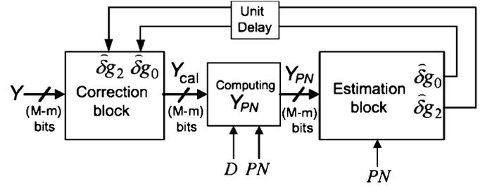
Fig. 5. Digital calibration unit for the second-order gain calibration of the pipeline stage in Fig. 4.
