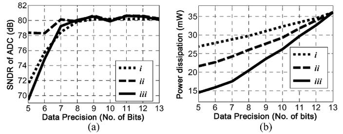
Fig. 6. (a) SNDR of the calibrated pipelined ADC based on MATLAB simulations and (b) the power dissipation of its digital calibration unit (Fig. 5) based on FPGA synthesis versus the following: *i*) number of bits in  $Y$ , with  $Y_{PN}$  having its full precision (13 bits); *ii*) number of bits in  $Y_{PN}$  having its full precision (13 bits); and *iii*) number of bits in  $Y_{PN}$  and  $Y$ .
