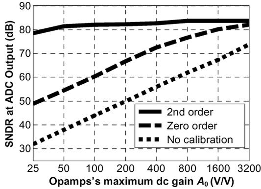
Fig. 3. SNDR versus opamp's maximum dc gain  $A_0$ , with no calibration, zero-order gain calibration [4], and second-order gain calibration [7].
