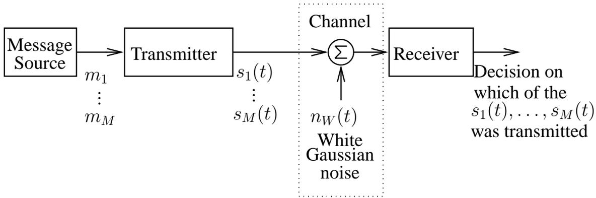
Figure 37: Digital transmission model
