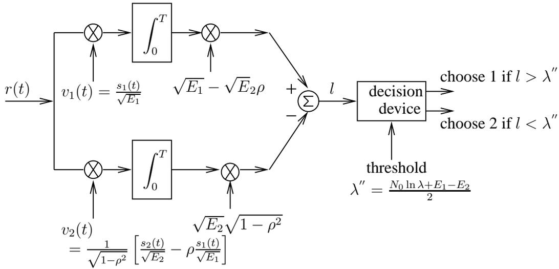
Figure 46: Optimal receiver (MAP receiver) for binary modulations (first implementation)
