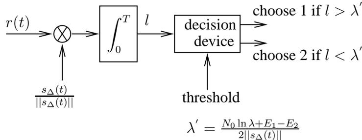
Figure 47: Optimal receiver (MAP receiver) for binary modulation (second implementation)
