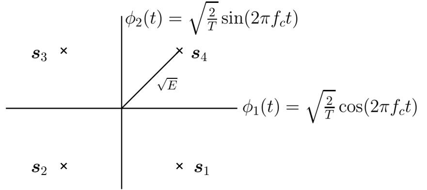
Figure 38: Signal space for QPSK
