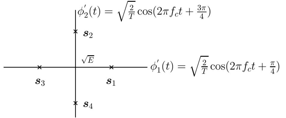
Figure 39: Rotated signal space for QPSK
