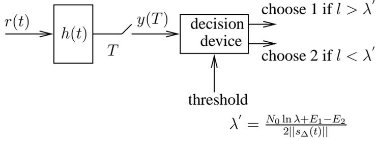
Figure 48: Optimal receiver (MAP receiver) for binary modulation (second implementation)
