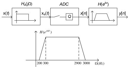
a) In designing a telephone system, a near-ideal analog anti-aliasing filter  $H_a(j\Omega)$  of bandwidth 4 KHz is used before the sampling circuit (such that the output of  $H_a(j\Omega)$  has no energy at frequencies above 4 KHz).
