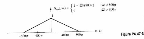
(a) If in Figure P4.47-1 the sampling rate is  $2\pi/T = 1600\pi$ , and the discrete-time system has frequency response
