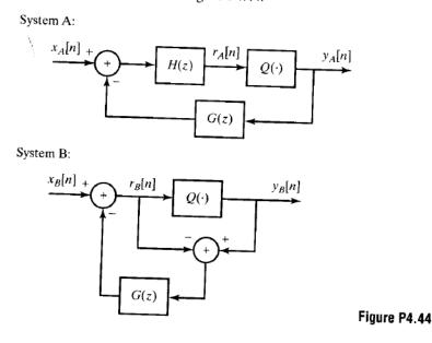
where  $Q(\cdot)$  represents a quantizer which is the same in both systems. For any given G(z), can H(z) always be specified so that the two systems are equivalent (i.e.,  $y_A[n] = y_B[n]$  when  $x_A[n] = x_B[n]$ ) for any arbitrary quantizer  $Q(\cdot)$ ? If so, specify H(z). If not, clearly explain your reasoning.
