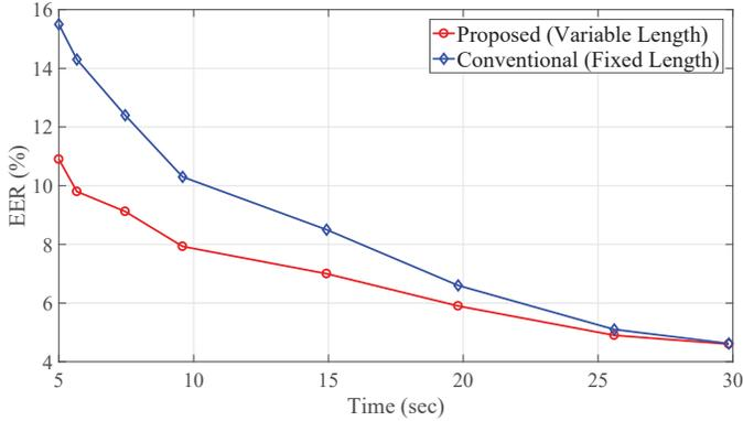
Fig. 5. ECG recognition performance. EER of ECG recognition using the proposed stopping criteria HC is compared with ECG recognition without HC stopping criteria, i.e. same recording length for all sessions.
