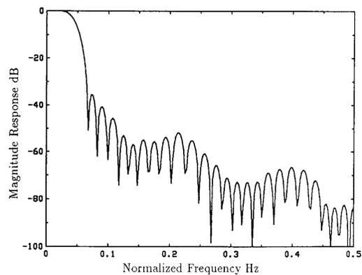
**Fig. 3** Magnitude response of the lowpass filter for system T4. The weighting factors are  $(\gamma_1, \gamma_2, \gamma_3, \gamma_4) = (100, 1, 1, 0.01)$ .
