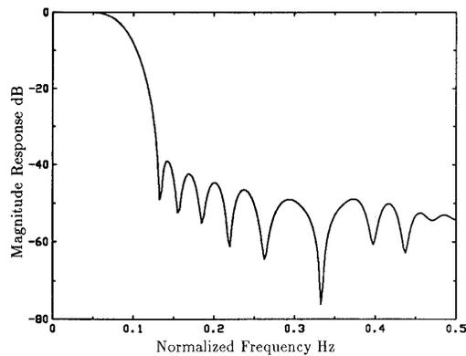
**Fig. 2** Magnitude response of the lowpass filter for system T3. The weighting factors are  $(\gamma_1, \gamma_2, \gamma_3, \gamma_4) = (100, 1, 1, 0.01)$ .
