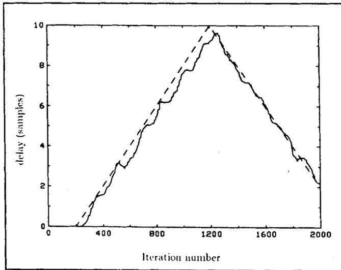
Figure 5: LMS adaptive delay response to a reference delay ramp of 0.01 sample/sampling period and for a 200-tap reference impulse response; dashed curve: reference delay;  $\mu = 0.01$ ,  $\alpha = 0.02$ . White Gaussian input.
