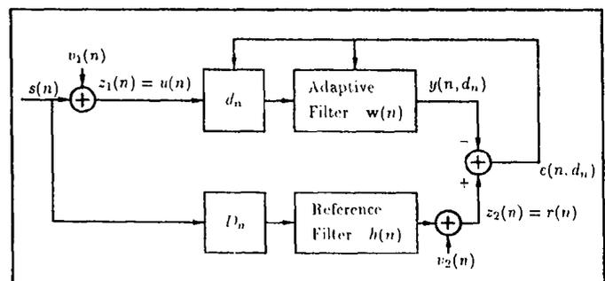
Figure 2: Systems identification configuration with the delays before the filters.
