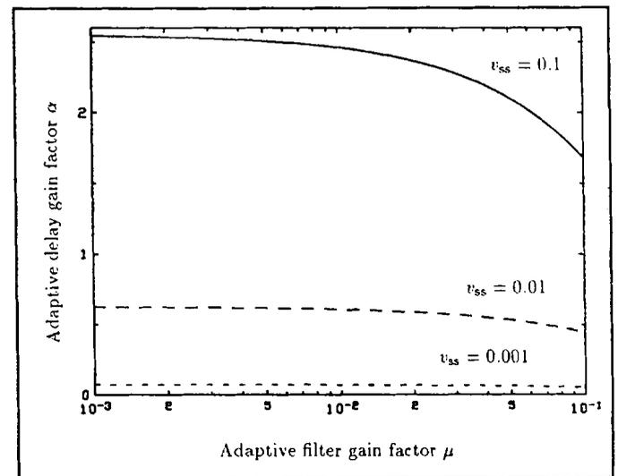
Figure 3: Theoretical curve of  $\alpha$  versus  $\mu$ ; SNR = 10 dB; small-dash curve:  $v_{ss} = 0.001$ ; large-dash curve:  $v_{ss} = 0.01$ ; continuous curve:  $v_{ss} = 0.1$ .
