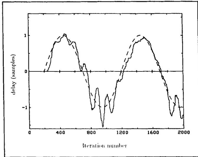
Figure 6: LMS adaptive delay response to a sinusoidal reference delay variation and for a 200-tap reference impulse response; dashed curve: reference delay;  $\mu = 0.01$ ,  $\alpha = 0.02$ . White Gaussian input.
