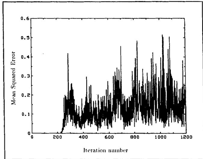
Figure 7: Learning curve for the joint algorithm coping with a reference delay ramp of 0.01 sample/sampling period (corresponding to Fig. 5);  $\mu = 0.01$ ,  $\alpha = 0.02$ .
