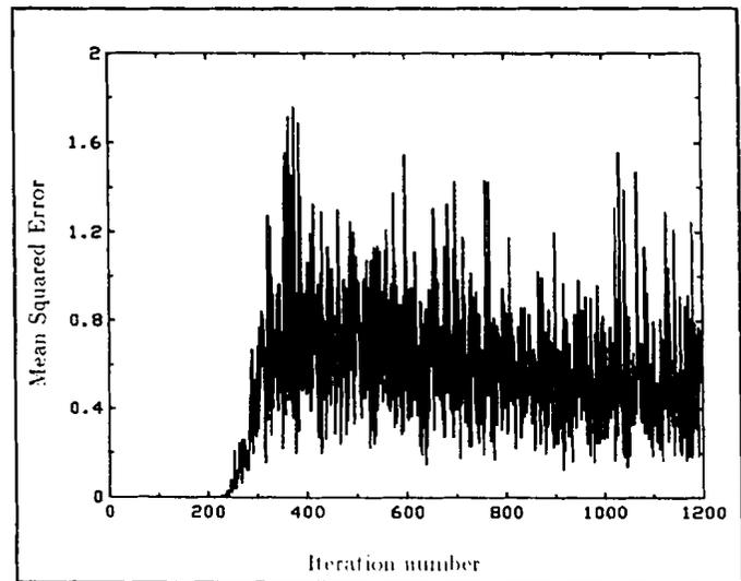
Figure 8: Learning curve for the single adaptive filter coping with a reference delay ramp of 0.01 sample/sampling period (note the scale difference compared to Fig. 7);  $\mu = 0.01$ . White Gaussian input.
