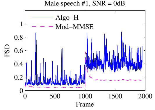
**Fig. 4.** FSD comparison between proposed noise PSD matrix estimation and algorithm from [8]
