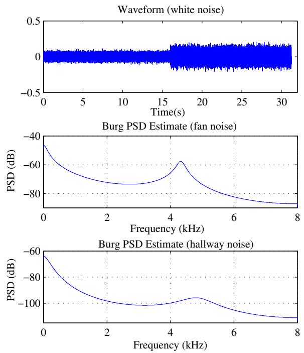
**Fig. 2.** Noise signals used in experiments. From top to bottom: non-stationary WGN, AC fan noise and hallway noise
