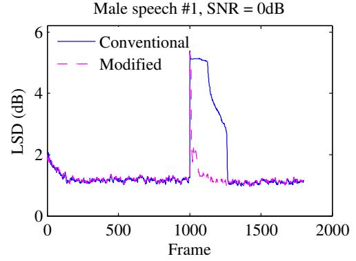
**Fig. 3.** LSD comparison between modified and conventional IMCRA algorithms for auto-PSD estimation
