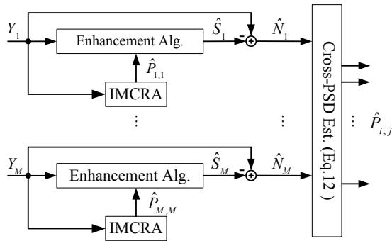
**Fig. 1.** Proposed cross-PSD estimator
